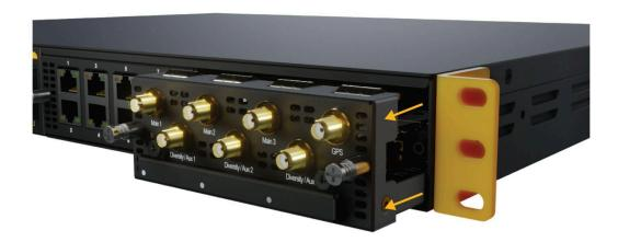
**Step 5**: Install the new module. Make sure it is correctly aligned and press the module firmly into place. The FlexModule should sit flush with surrounding FlexModules or slightly countersunk (1-2mm) of the router chassis.
